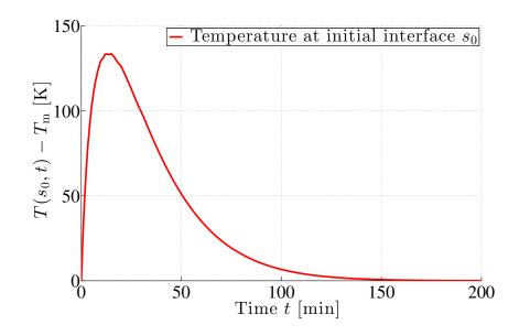
Temperature warms up and cool into melting point
